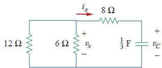
Đs:  $45e^{-0.25t} \text{ V}, 15e^{-0.25t} \text{ V}, -3.75e^{-0.25t} \text{ A}$ .
