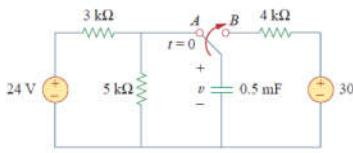
$$v(0^-) = \frac{5}{5+3}(24) = 15 \text{ V} \quad v(0) = v(0^-) = v(0^+) = 15 \text{ V}$$
